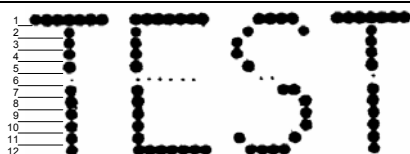
Adjusting screw is turned 10 minutes counterclockwise
