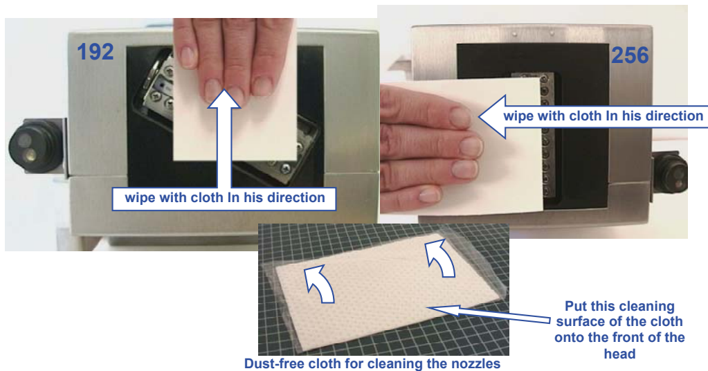
Fig. 6.2.2. Wiping the front of the print head (where the nozzles are) with dust-free cloth
